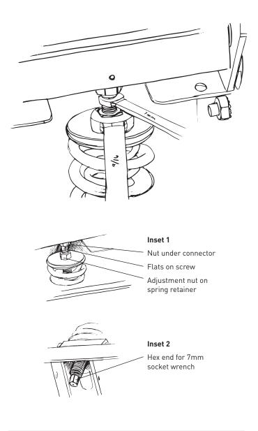
TOOLS REQUIRED: 7MM (9/32 INCH) OPEN END WRENCH OR 7MM (9/32 INCH) SOCKET WRENCH, DEPENDING ON THE MODEL AND 9/16 INCH OPEN END WRENCH (OR 14MM OPEN END WRENCH MAY WORK)
