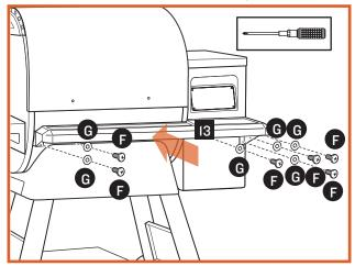
**INSTALL HANDLE AND GREASE PAN WITH LINER**
